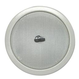
The EMCS-803 6.5" Loudspeaker offers high quality performance and wide frequency response. The speaker consists of a 6" diameter dual cone type with power rating of 6 watts. The wide range of the frequency which produces a sound quality with low distortion. The frequency response of this speaker is in the range from 45Hz to 18KHz resulting in a wide uniform coverage of 120 degrees thereby producing an excellent sound reproduction for vocal and music for a wider coverage area.
